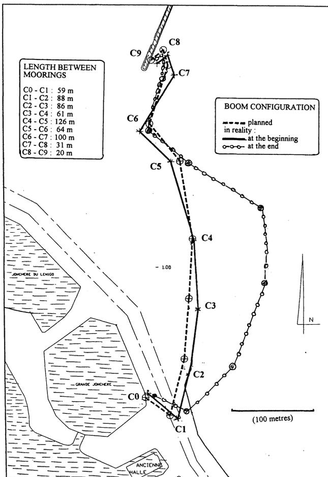
Figure 2. Evolution of the boom configuration
